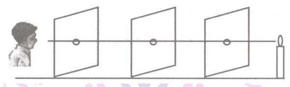
candle is seen effortlessly. Now, the middle one of the three cardboards is displaced from its position. Now, we are unable to see the light. The reason behind this is that the light travelling in the straight line is obstructed due the misalignment of the cardboards. This proves that light always travels in a straight line.
