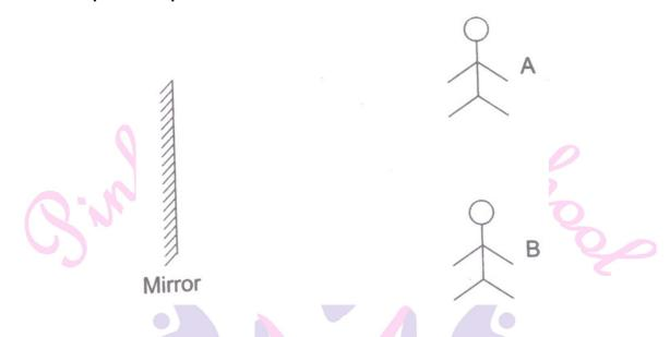
The light rays from A falls on the mirror and gets reflected and reaches B, the light from B falls on the mirror and reflects on A. The path of light is just reversed as shown in the figure.
