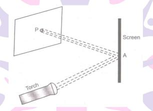
The material of this sheet is transparent glass Torch which allows the light to pass and the patch of light is obtained on screen.
