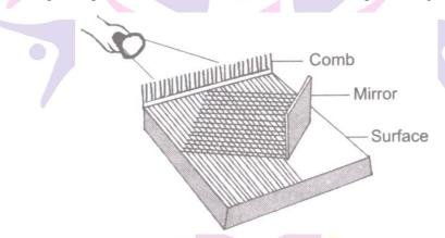
Light travels in straight line and gets reflected from a mirror.
