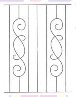
The photograph given as Fig. above shows a section of a grille made up of straight and curved iron bars. How would you measure the length of the bars of this section, so that the payment could be made to the contractor?
