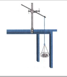
Note down the total weight required to break the thread. This indicates the strength of the fibre.
